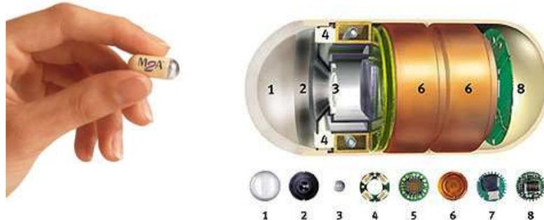
**Figure 1.1:** The M2A© camera (left) and the camera components (right) [15].
